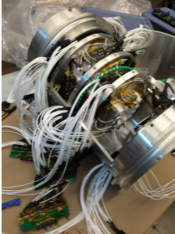
Figure 2.9: Fully cabled FAUST. The green board in the bottom left is an adapter board, which contains traces to combine the raw signals from four DADL detectors into a 34-pin header to go through feedthroughs in the FAUST chamber faceplate.
