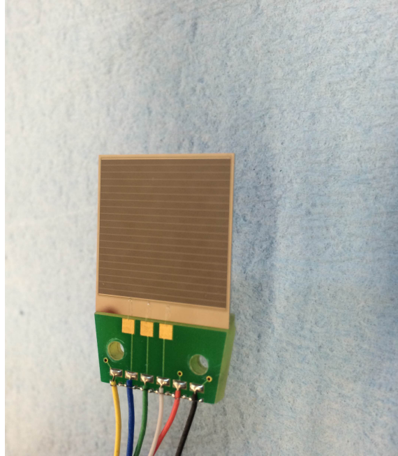
Figure 2.6: Representative DADL silicon detector. As indicated by the horizontal stripes, the charge is split in the vertical dimension on the front of the detector. Signalling across the bottom is as shown in Table 2.5
