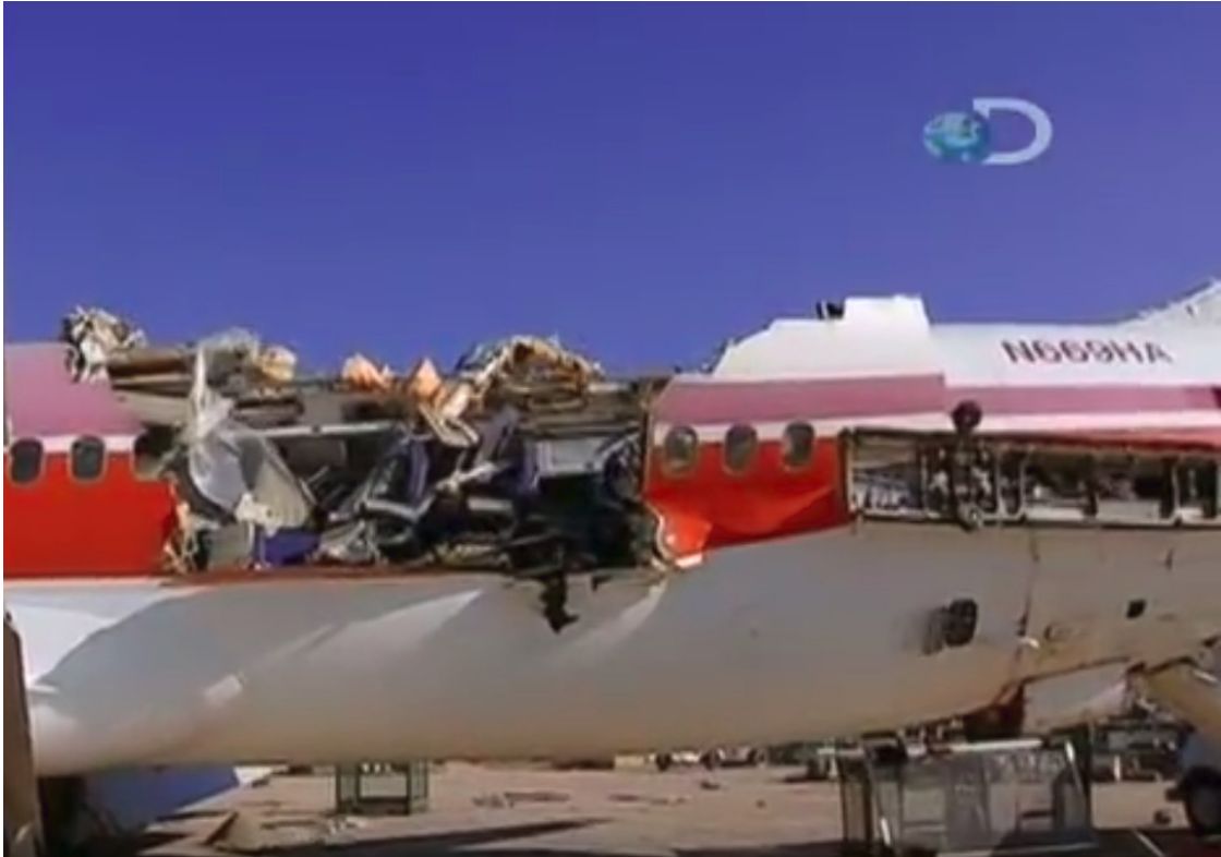
Figure 3.4: Explosion by a large explosive charge by a MythBusters' experiment. For video, see https://youtu.be/Fi1_117M8FA?t=4m17s
