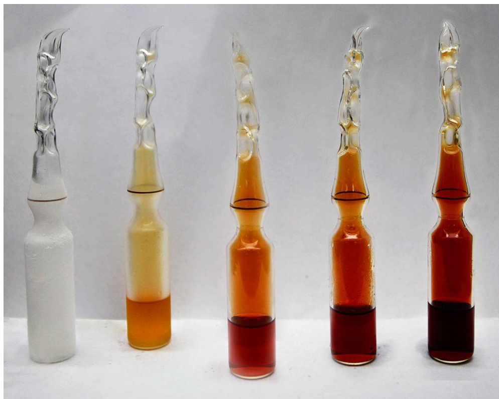
Figure 43 Overlaid pictures taken to the same sealed ampule containing 99.9% pure \text{NO}_2/\text{N}_2\text{O}_4 at different temperatures. From left to right -196\text{ C} , 0\text{ C} , 23\text{ C} , 35\text{ C} , 50\text{ C} . © Efram Goldberg / CC-BY-SA-3.0
