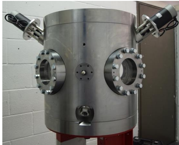
Figure 26 Turbulent flame bomb during assembly. Plumbing and wiring work is missing in this picture.
