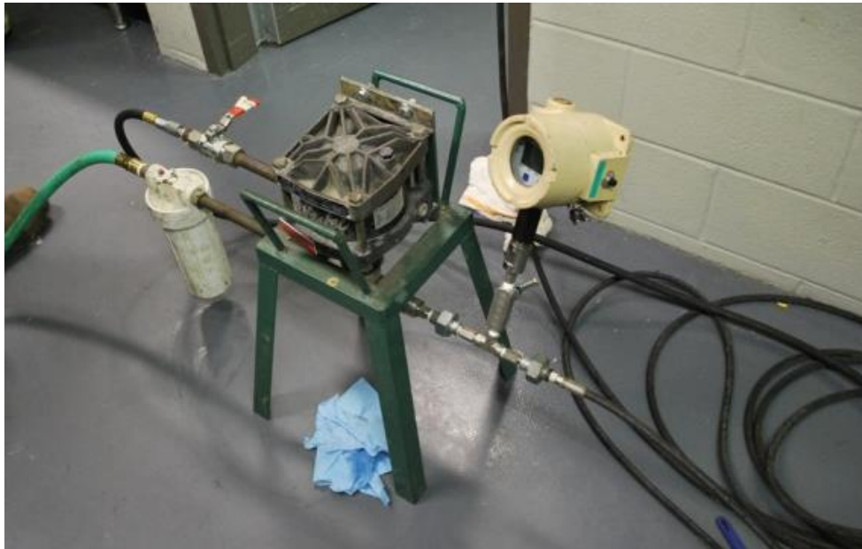
Figure 35 Pneumatic pump and pressure transducer with data log
