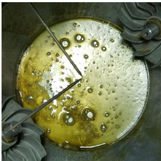
Figure 42 Water condensed inside the bomb after 10-bar experiment. The oxidizer was air ( O_2:N_2::1.0:3.76 ). Hydrogen was burned at \phi=0.5 . Top view.
