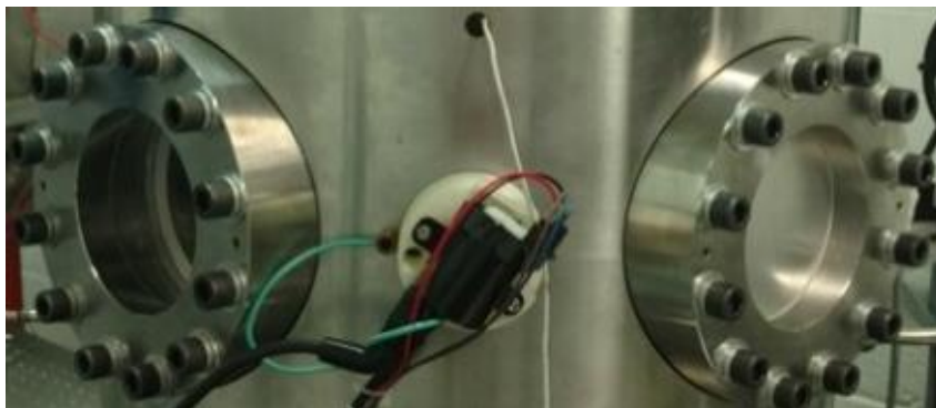
Figure 39 The quartz substrate (left) been substituted by aluminum blank (right).
