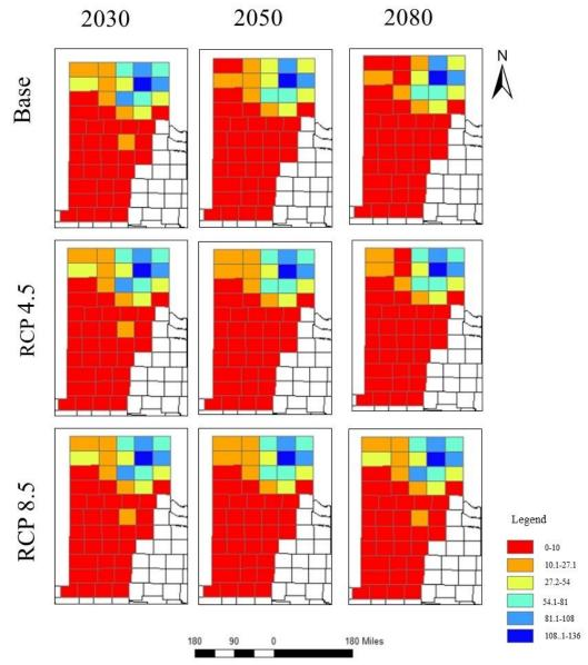
Figure 3.8: Average saturated thickness in the Ogallala aquifer by county in the Texas High Plains in 2030, 2050, and 2080 under the base, RCP 4.5 and RCP 8.5 scenarios.
