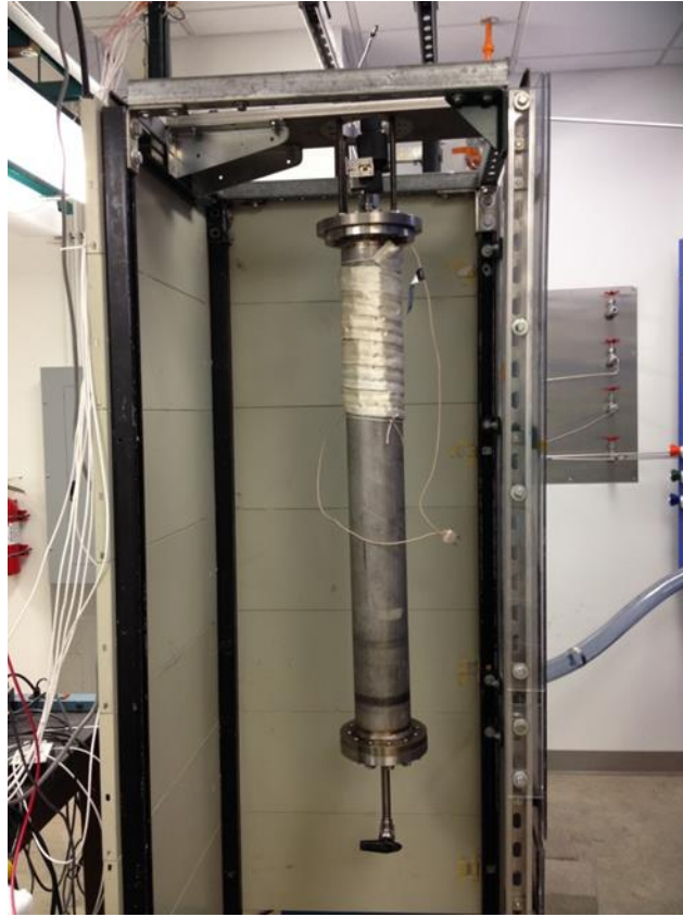
Figure 20 Reaction vessel mounted in the safety enclosure
