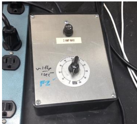
Figure 14 Variable voltage controller
