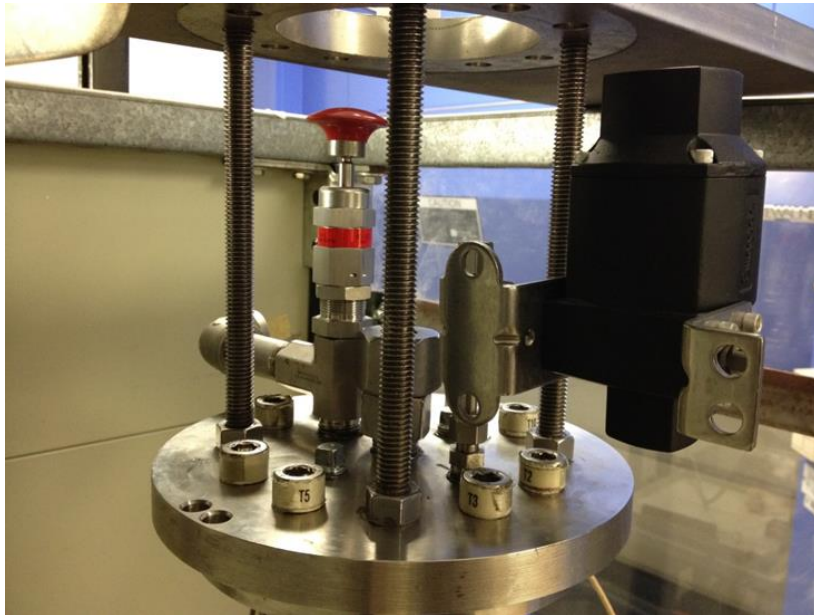
Figure 17 Top flange and line connections
