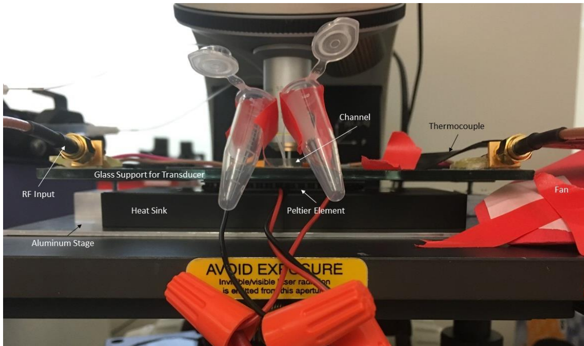
Fig. 20 Side view of the transducer setup under the microscope with temperature regulation components.
