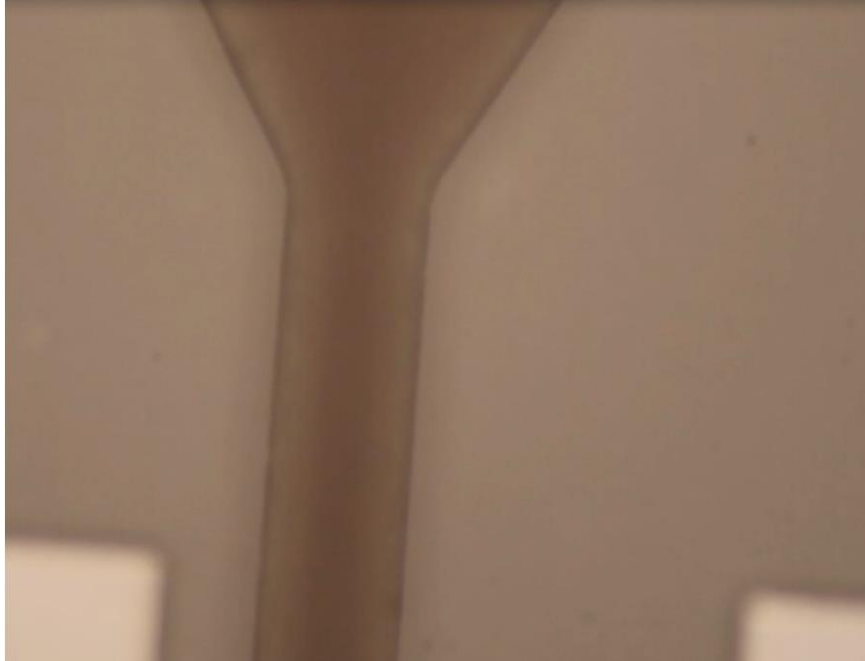
Fig. 34 Laminar streams of blood and PBS shown at the exit trifurcation of a 25 mm long channel with flow rates of 0.25 and 5 \mu\text{L}/\text{min} for blood and PBS, respectively. Undiluted whole blood is placed in the central stream and sheathed by two PBS streams. Significant diffusion of blood cells was observed due to reduced flow rates and increased channel length compared with the experiment shown in Fig. 33. The main channel width was 150 \mu\text{m} . The pillar structure width was 600 \mu\text{m} .
