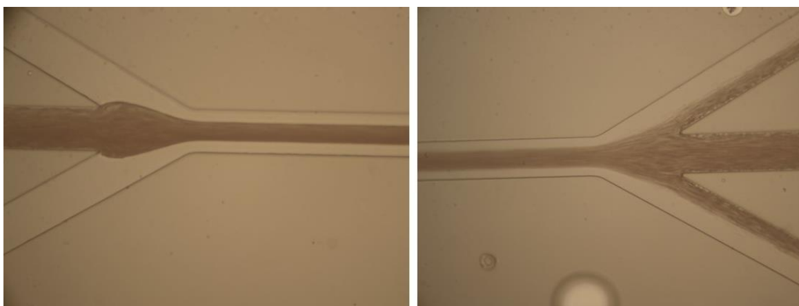
Fig. 33 Example of flow set up for acoustic experiment, showing the entrance (left) and exit (right) of the microfluidic channel with the transducer off. Undiluted whole blood is placed in the central stream and sheathed by two PBS streams. Flow rates of 3 and 10 \mu\text{L}/\text{min} were used for blood and PBS, respectively. The channel length selected for final blood separation experiments was 15 mm between the two junctions. No significant diffusion of blood cells was observed. The main channel width and height were 150 \mu\text{m} and 50 \mu\text{m} , respectively.
