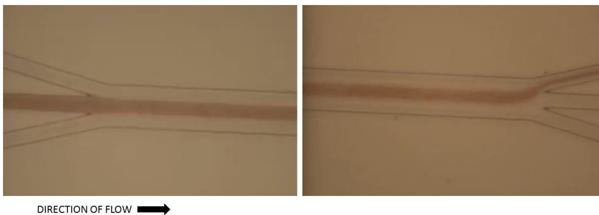
Fig. 47 Laminar streams in a trifurcated microchannel with 10% whole blood nanoparticle solution located in the sample stream and PBS used as the sheath fluid. At the exit from the main channel (right), a small amount of diffusion of the sample stream is seen compared with the entrance to the channel (left). Flow rates were 3 and 10 \mu\text{L}/\text{min} for the 10% whole blood nanoparticle solution and PBS, respectively.
