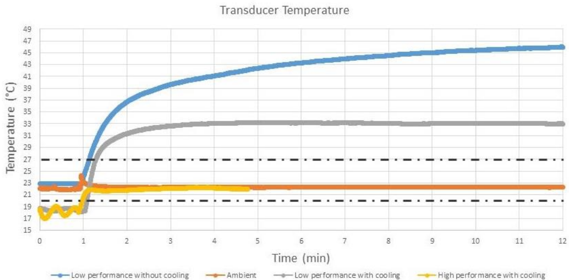
Fig. 36 With the addition of the cooling system, the transducer temperature was controlled, although it plateaued above the set point. Yellow and gray curves are examples of how the transducer temperature could be controlled with the cooling system. The blue curve shows that the transducer temperature continued to rise over time without use of the cooling system. The dashed lines indicate the temperature range where high performance blood separation was achieved and maintained. After using a transducer for several weeks, blood separation performance declined and in some experiments the heat produced increased. The gray and blue curves shows the transducer temperature with and without the cooling system when the blood separation was not maintained and had reduced performance from previous experiments. The orange curve represents the room temperature.
