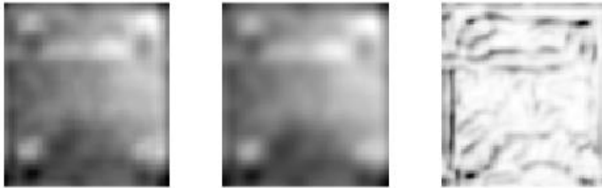
Figure VII.10 Comparison the estimated heat flux distribution from RPHF (mid) with original heat flux for simulation (left) by using image structural similarity index (right)
