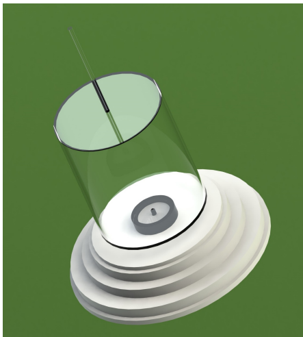
Figure IV.8: Schematic of the alignment configuration used to hold the sample cell during packing
