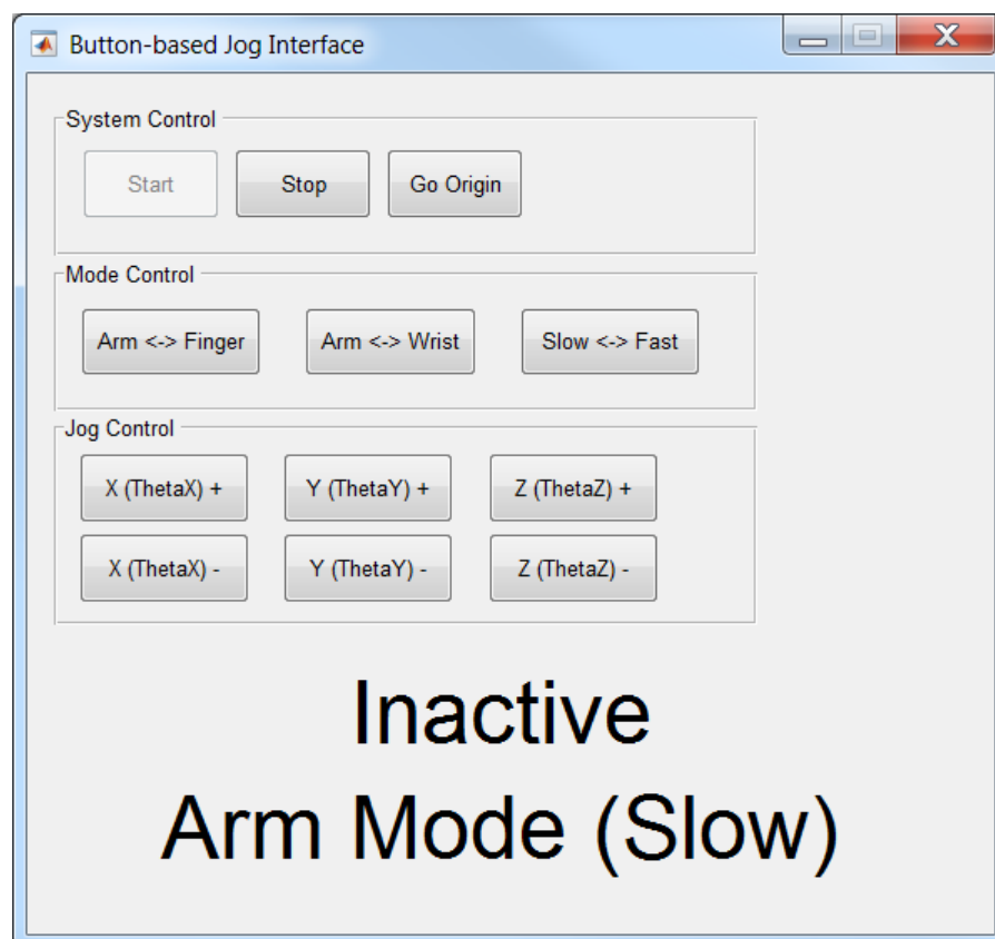
Figure 30 GUI button-based jog interface made by Matlab GUI
