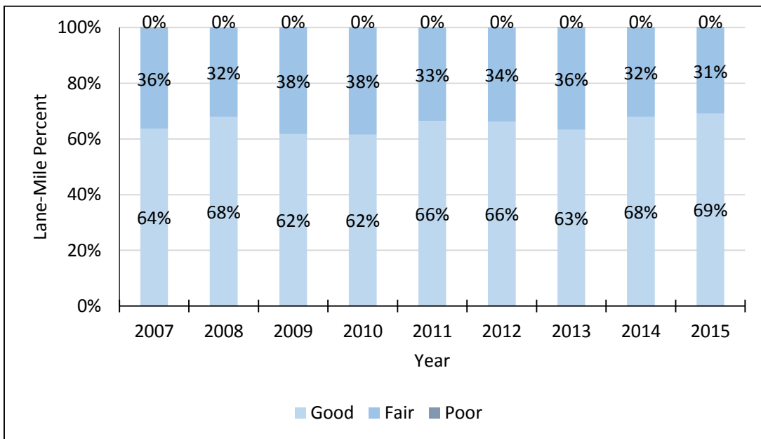
Figure 25-Performance of Rural Roads in the Houston District Based on IRI Thresholds Proposed in the January 2015 NPRM of MAP-21
