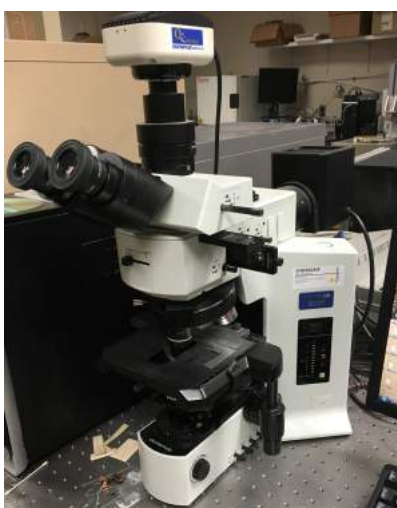
Figure 4-4 Optical microscope set-up with polarizer and analyzer lenses
