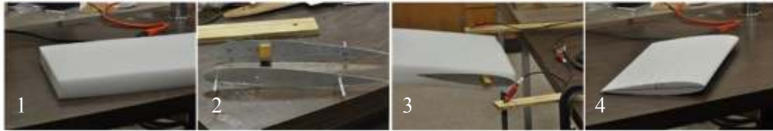
Figure 110. Shaping the airfoil - sequence of fabrication images showing: 1) initial form, 2) airfoil forms, 3) hot wire cutting, and 4) cut foam airfoil.
