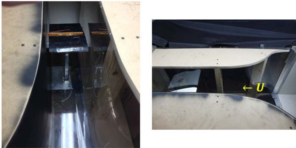
Figure 118. Converging inserts used to increase free stream velocity and mitigate edge effects when using 0.18 m span airfoils in the test section. a) Front view b) Side view.
