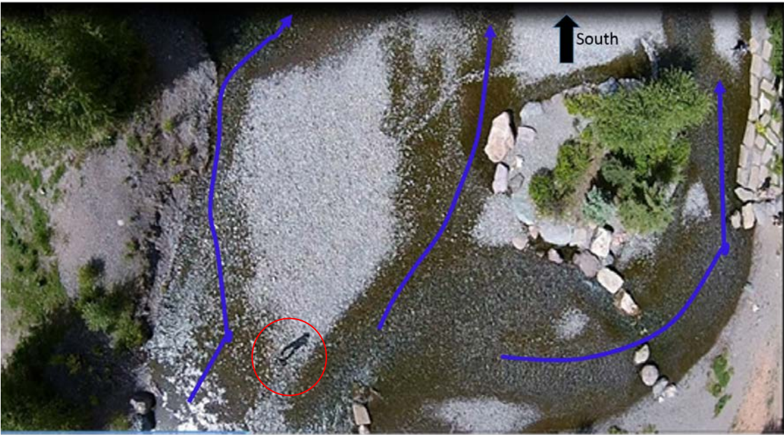
Figure 22: Flow paths in Instream Sedimentation Basin, 2014: Screenshot from UAV video, 6-foot shadow of field assistant for scale.
