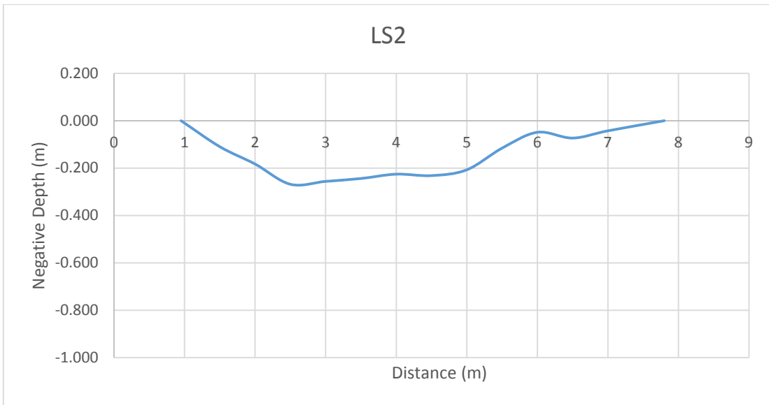
Figure A6: Channel bed geometry at waypoint LS2 (N 37°56.106, W 107°48.285), ~ 50 meters downstream of Laurel Street
