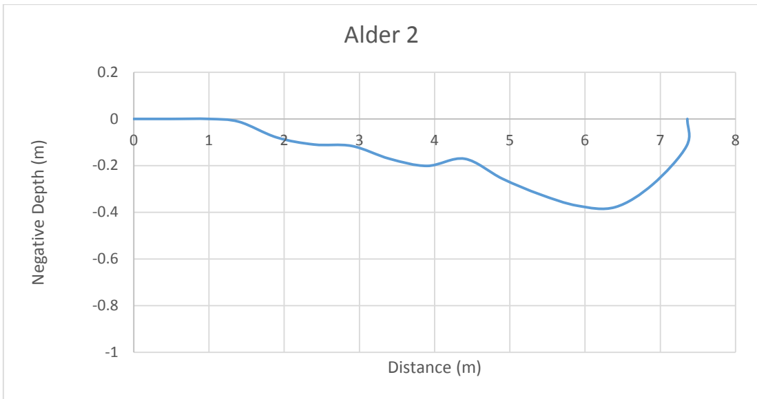
Figure A14: Channel bed geometry at waypoint ALD2 (N 37°56.127, W 107°48.495), 50 meters downstream of North Alder Street, just below Pacific Ave Bridge
