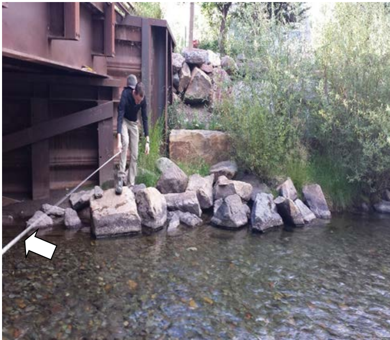
Figure 14: Photographs of performing a cross-section: a) Example of cross-section measurement using measuring tape; b) Field assistant (1.8 m, 6 ft. tall) measuring bank-to-bank width, holding measuring tape (denoted by arrow). Image taken from midstream.
