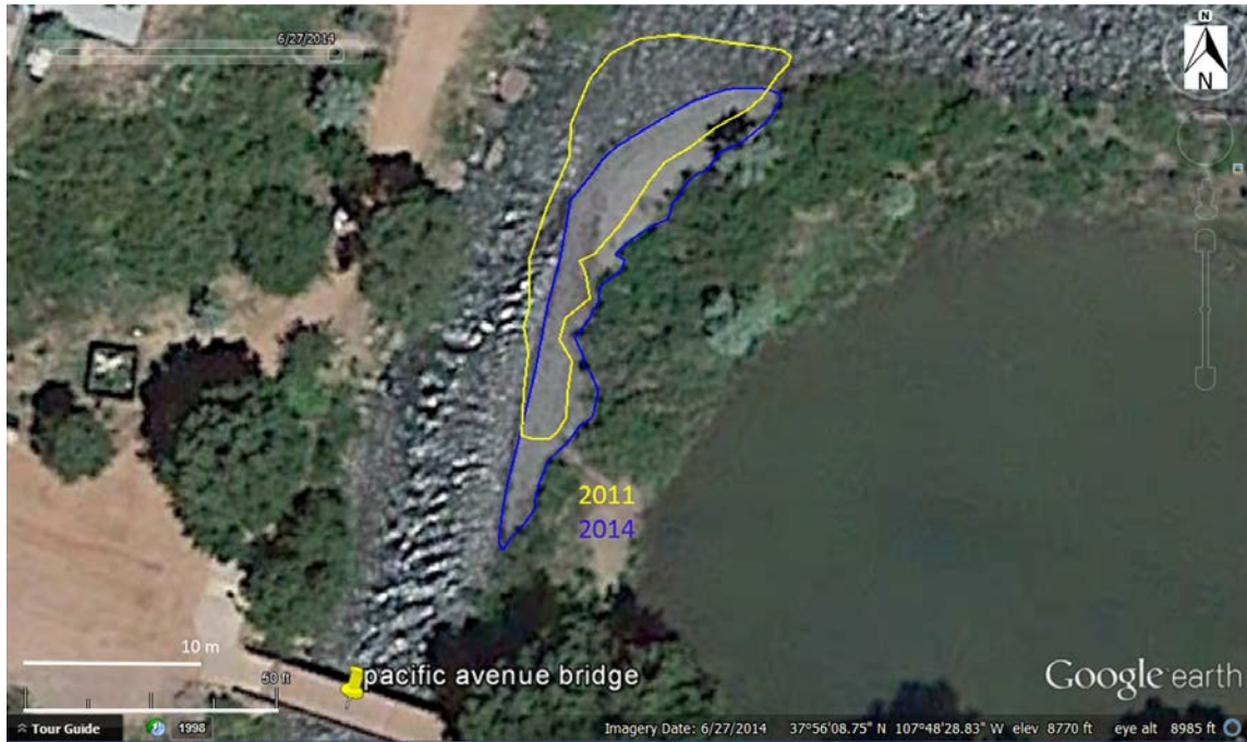
Figure 17: Changes in point bar sizes along the San Miguel River, upstream of Pacific Avenue Bridge. Point bar outlines from 2011 and 2014 are shown in yellow and blue respectively. Base is Google Earth® Image from 06/27/2014
