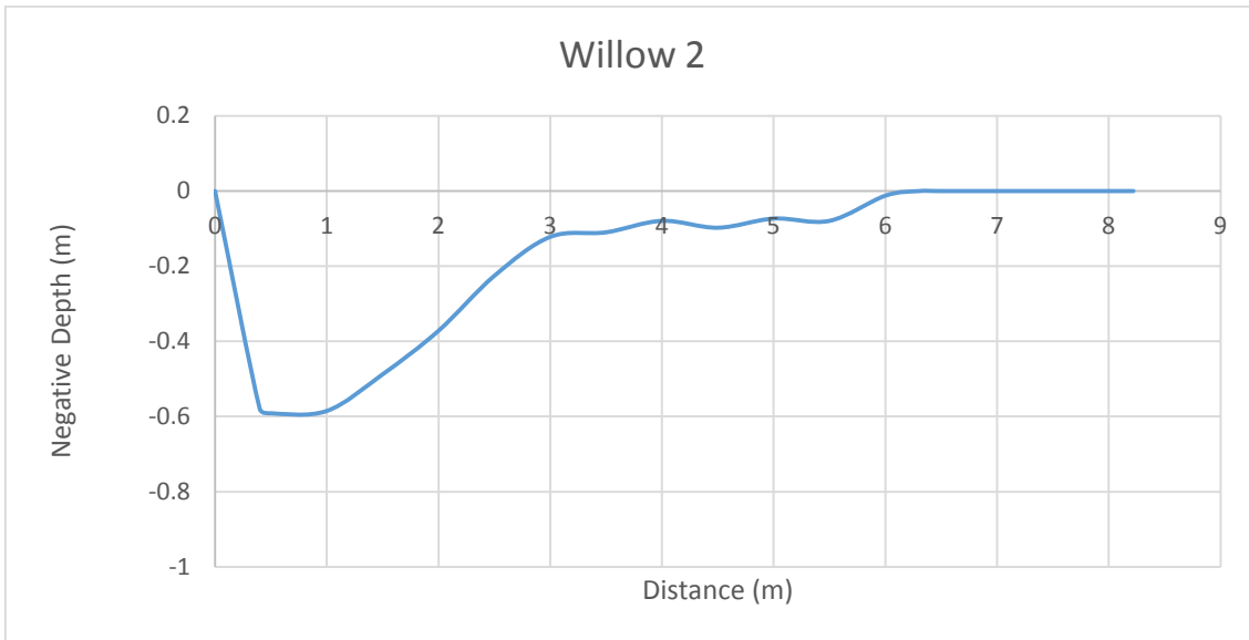
Figure A17: Channel bed geometry at waypoint WIL2 (N 37°56.102, W 107°48.588), ~ halfway between South Willow Street and South Spruce Street
