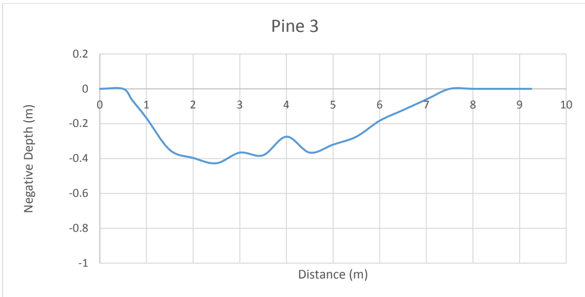
Figure A22: Channel bed geometry at waypoint PINE3 (N 37°56.100, W 107°48.753), ~ 70 meters downstream of Pine Street Bridge.
