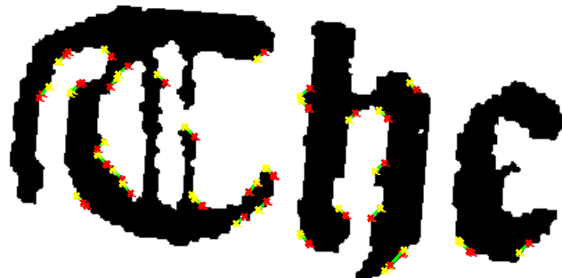
Figure 19: An example of Hough transform applied to a word image. Here, the green line segments are the detected angled straight lines.
