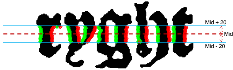
Figure 18: An example showing an intermediate step in the calculation of mean and IQR character width.
