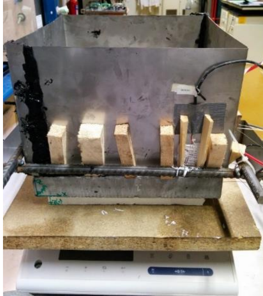
Figure 35: Experimental setup for rough surface concrete base in the lab
