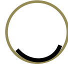
Fig. 5.3b—End view of sinusoidally buckled tubing string segment lying in a straight section of the wellbore
