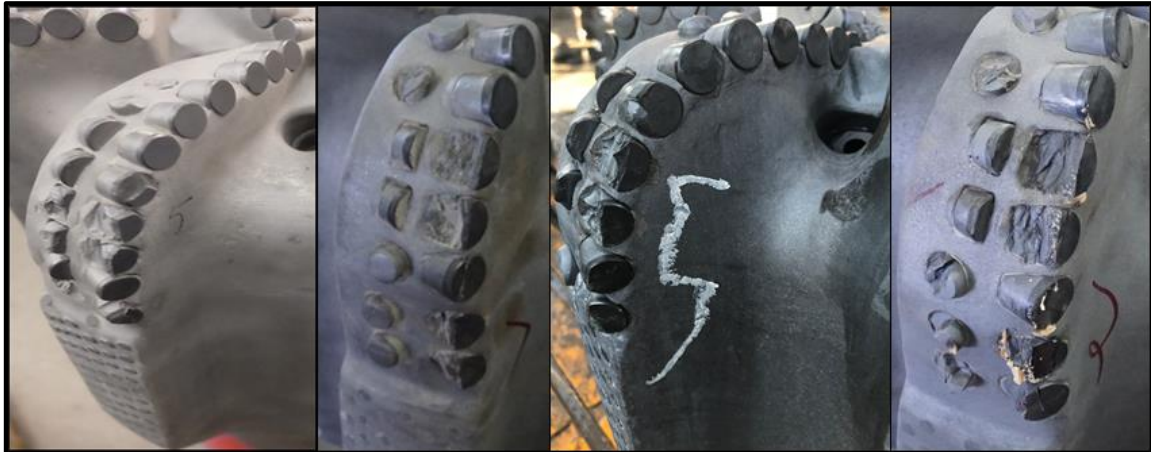
Figure 17 – Example of bits that had tangential overload of the gauge and shoulder cutters with no damage to the nose. Numbers on blade correspond to blade number, not well number.
