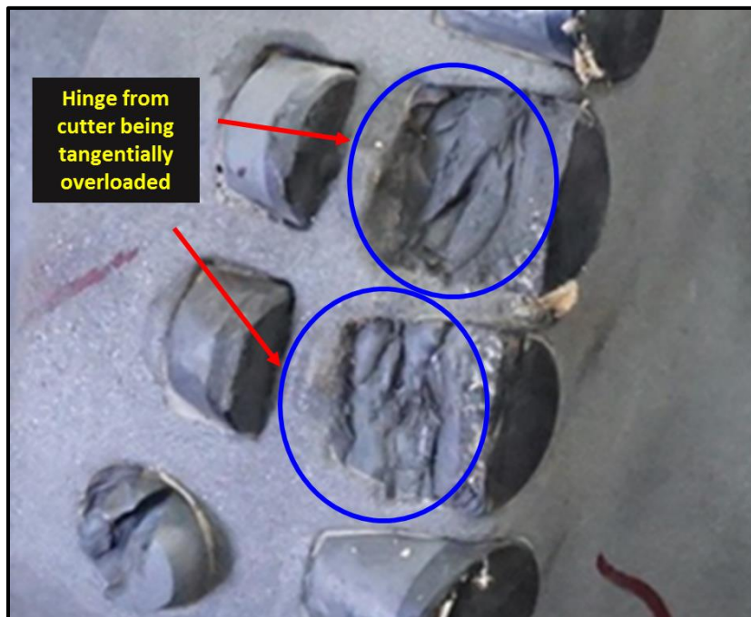
Figure 6 – Picture of typical tangential (hinge) failure that occurs on the trim and gauge cutters when drilling out of high-strength laminations.
