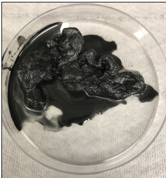
Figure 18. Graphene coated cotton after 12 hour reaction of DMF in graphene and diamine cellulose.
