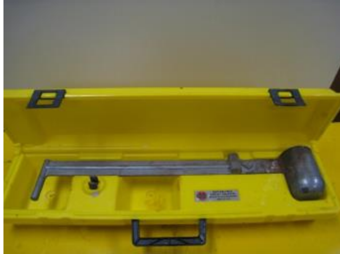
Figure 28. Baroid Mud Balance Model 140.
