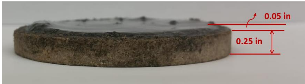
Figure 49. Filter cake thickness formed by MOBDF A at 140°F/300 psi.
