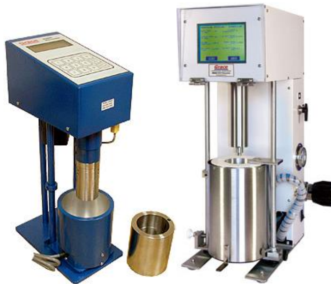
Figure 27. (Left) Grace M3600 Viscometer. (Right) Grace M5600 HP/HT Rheometer.
