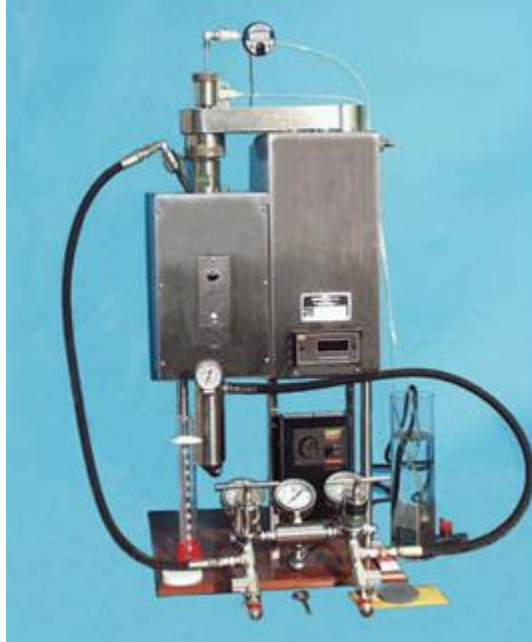
Figure 30. OFITE Dynamic HP/HT Filter Press.
