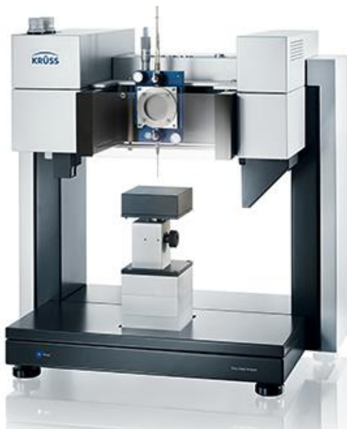
Figure 33. Kross Drop shape analyzer (DSA 100).
