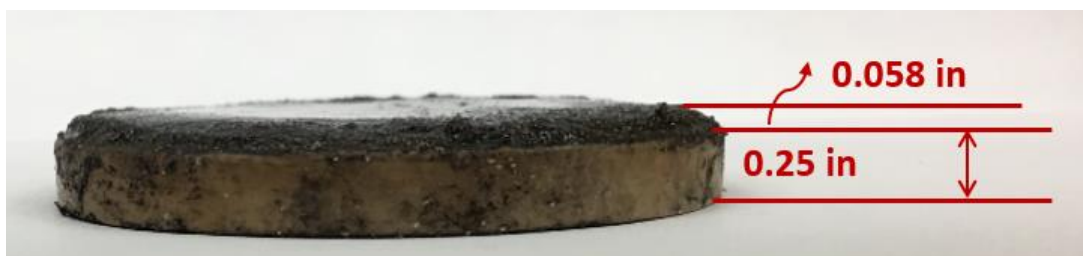
Figure 53. Filter cake thickness formed by MOBDF B at 190°F/300 psi.
