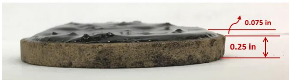
Figure 51. Filter cake thickness formed by MOBDF A at 250°F/500 psi.
