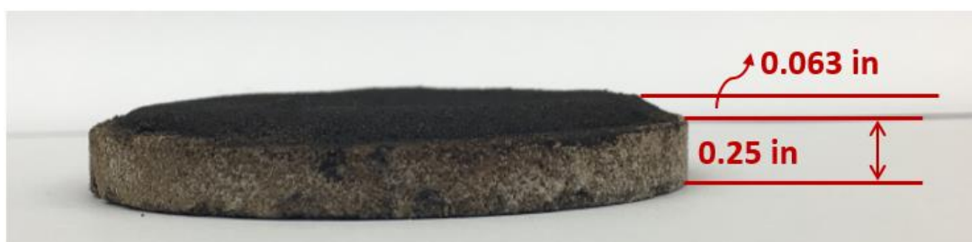
Figure 52. Filter cake thickness formed by MOBDF B at 140°F/300 psi.
