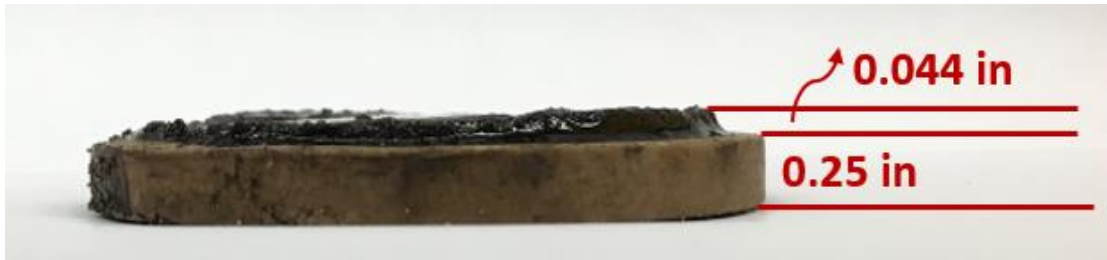
Figure 54. Filter cake thickness formed by MOBDF B at 250°F/500 psi.
