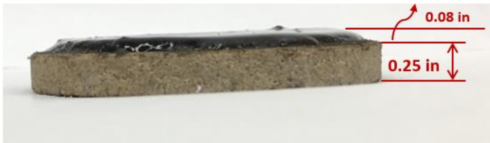
Figure 50. Filter cake thickness formed by MOBDF A at 190°F/300 psi.
