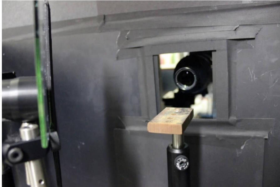
Figure 9. Close-up of propellant strand holder, DIH lens placed behind a protective window, and collimating lens behind protective window.
