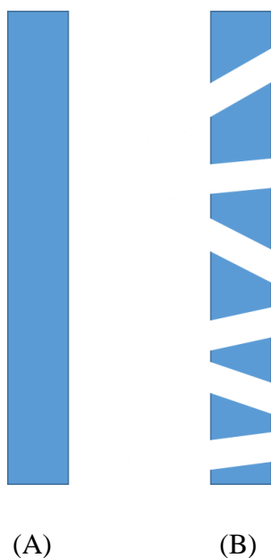
Figure 3. Schematic showing the side angle of a holographic film. (A) Holographic film that has not been exposed yet. (B) Holographic film that has been exposed.
