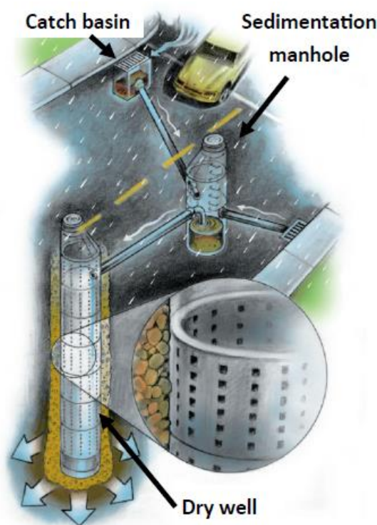
Figure 2. Typical city dry wells system in Portland (Reprinted from OEHHA 2018)
