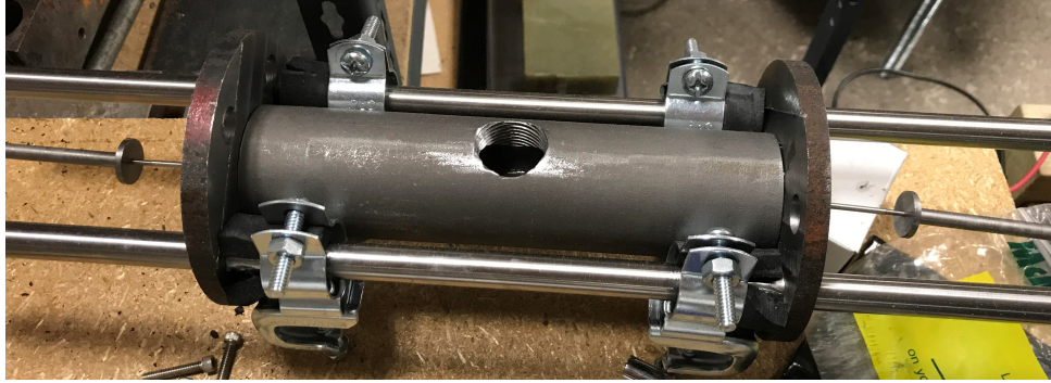
Figure 2.18: The manufactured and assembled shaker.
