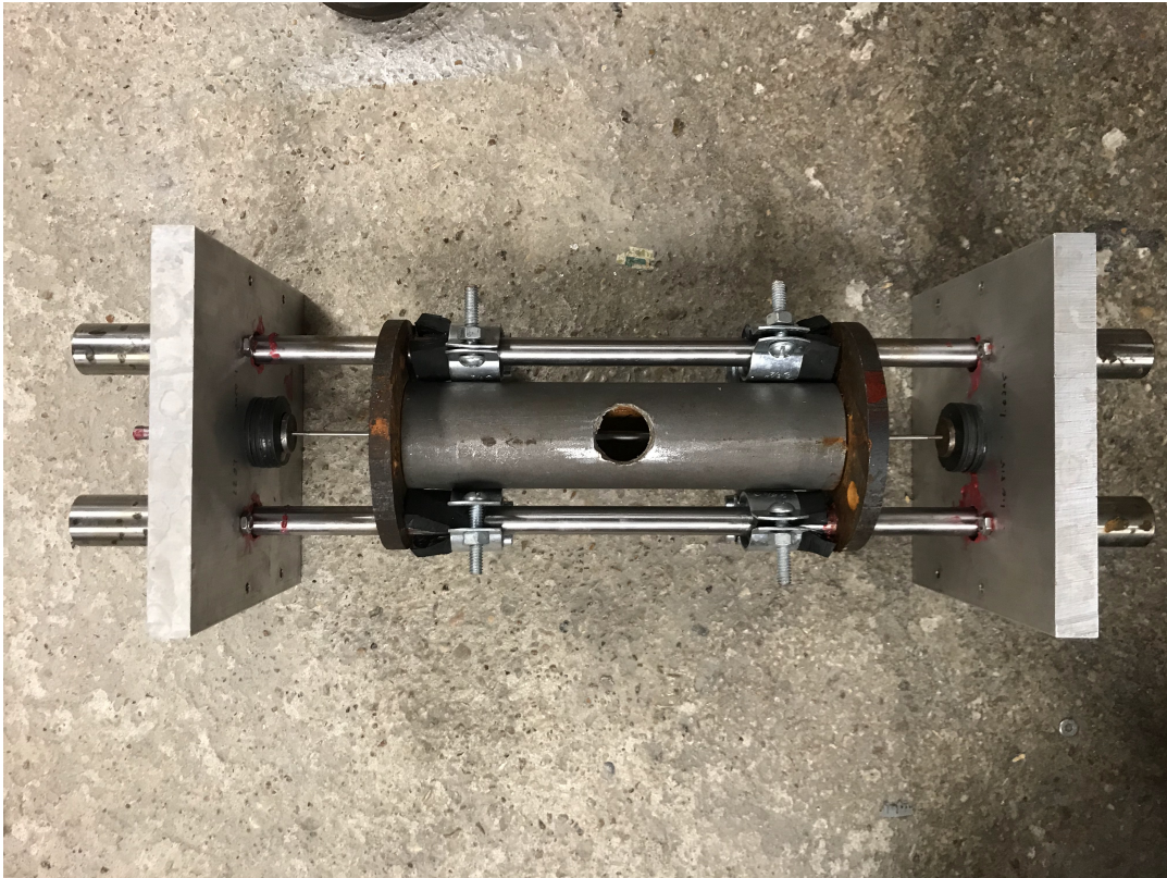
Figure 2.24: The shaker being tested for shaft misalignment
