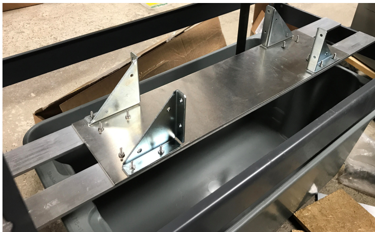
Figure 2.21: The manufactured and assembled shaker base sitting over the reservoir.
