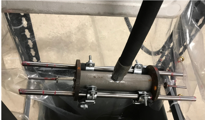
Figure 3.10: Shaker hanging by the hose, before the preliminary flow test
