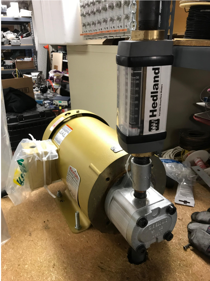
Figure 2.16: Bosch Rexroth gear pump and induction motor used for experiments.
