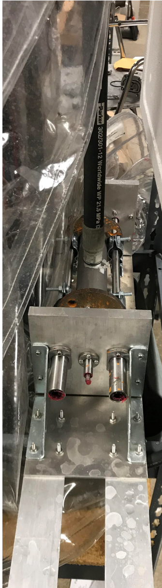
Figure 2.22: The assembled shaker and base sitting on the rig, with shielding curtain pulled back.
