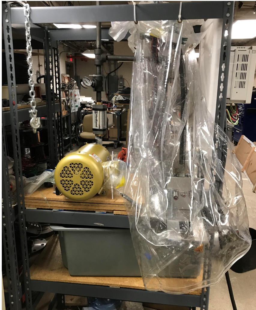
Figure 2.23: The fully assembled test rig, with shielding curtain to protect the motor from the water sprayed by the shaker
