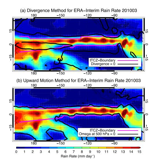
Figure 2.5: (a) Identifying ITCZ boundaries by finding where the 1000-850 hPa layer mean divergence and (b) vertical pressure velocity at 500 hPa equal zero (black); results are compared against the rain rate threshold methodology (magenta).
