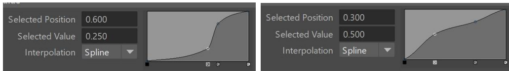
Figure 24: The effect of changing the ease-in points position along the remap curve. The first shows a change in percent while the second shows a change in value.
