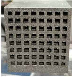
Figure 1. Frontal view of manufactured 8 x 8 x 8 lattice.
