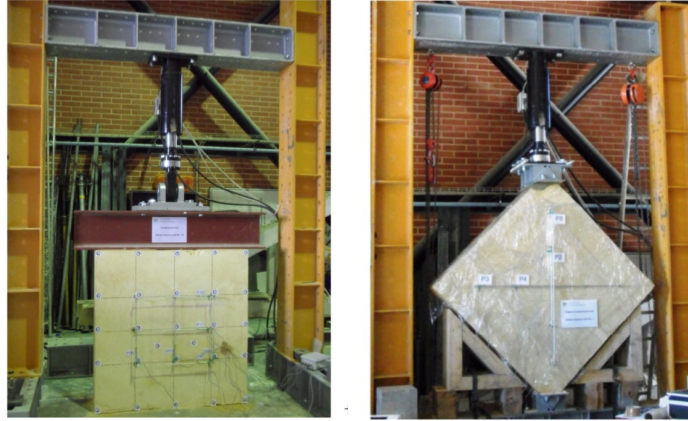
Figure 1.3. Typical tests on adobe masonry. A) Simple compression. B) Diagonal compression (Reprinted from Blondet, M. et al. 2015).
