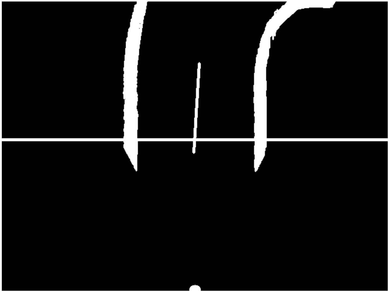
Figure 4.7: Overhead perspective of the Hough line transformed track from Figure 3.5, with search line (horizontal line) and navigation trajectory (vertical middle line) projected onto the image
