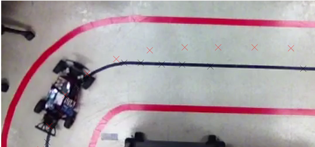
Figure 5.5: Vehicle navigating through the second turn and small straightaway of the track with center line reference points (black) and actual travel points (red)
