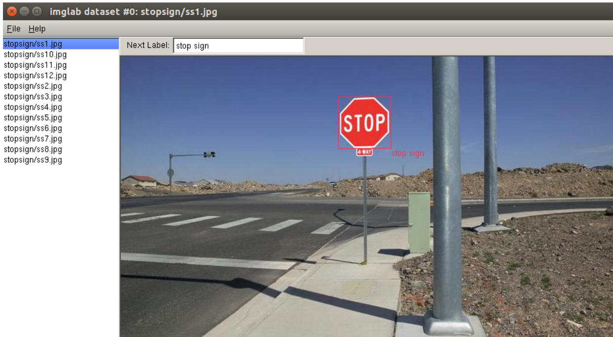
Figure 4.8: User interface for the imglab tool used for training stop sign and speed limit sign SVM
