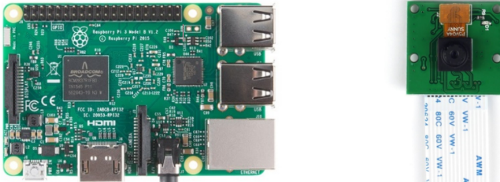
Figure 2.3: Raspberry Pi 3 Model B (left) and Arducam 5 Megapixel Camera (right) [21],[22]
