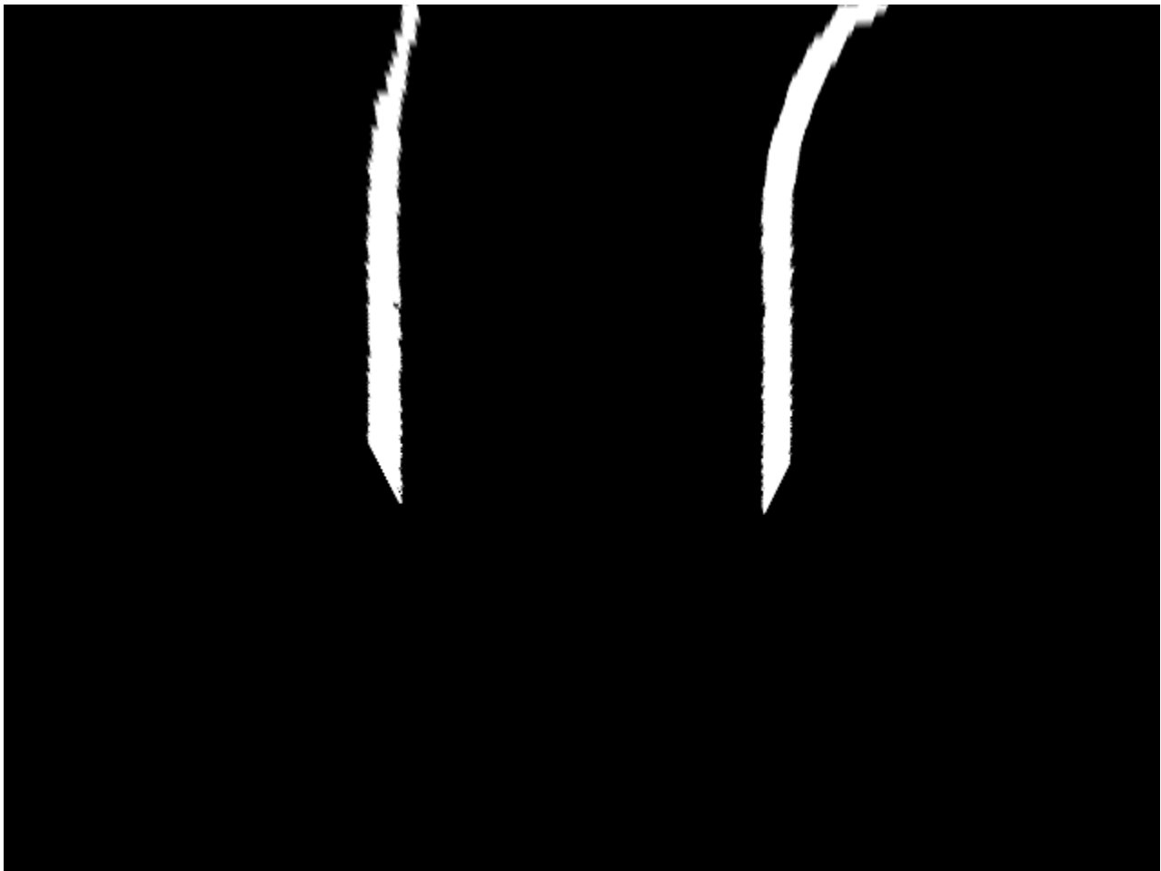
Figure 4.6: Overhead perspective transformed image of Figure 4.2, showing how the track appears from straight above
