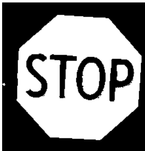
Figure 1.7: Color masking performed on a stop sign, with white pixels indicating retained pixels, and all other pixels rejected
