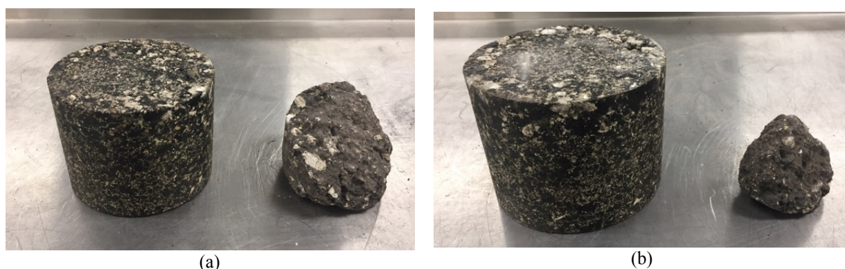
Figure 72. Specimens Before and After Cantabro Abrasion Loss Test; (a) Mixture C-80L-LF and (b) Mixture C-60L-GF
