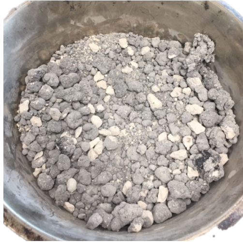
Figure 60. Appearance of Foamed Cold Recycled Mixture with 3% Foamed Binder and No MC after Mixing
