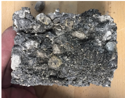
Figure 62. Cross Section of Foamed Cold Recycled Mixture Trial Specimen with 4% Foamed Binder Content and 4% MC
