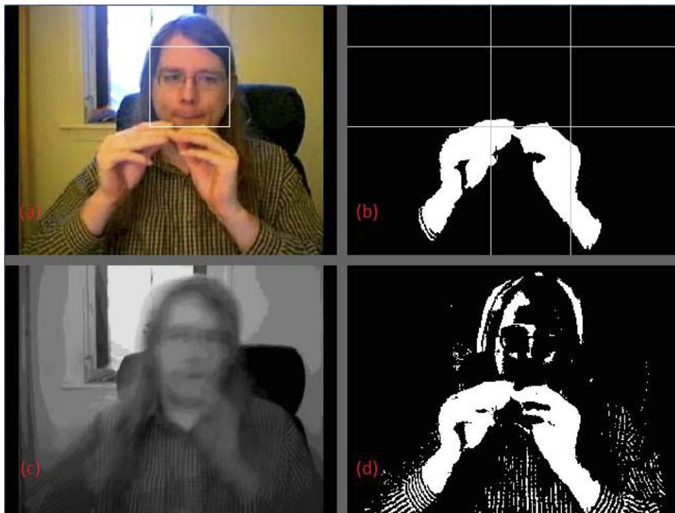
Figure 2. Steps involved in performing background-foreground separation. (a) is the incoming frame of the video; (b) is the final compute foreground; (c) is the background model used for thresholding the incoming frame; and (d) is the foreground image after thresholding but before the morphological opening.
