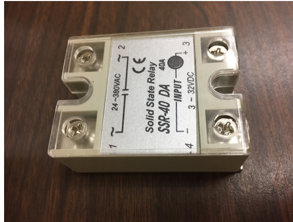
Figure 5.16: A 40A solid state relay used in the control box.
