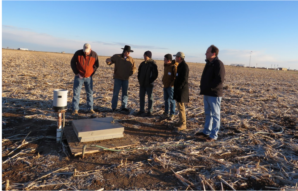
Figure 2.25: Surface appearance of a monolithic weighing lysimeter.
