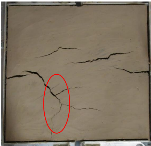
at maximum tensile force, after 19.5-hour, w = 32.9\%
