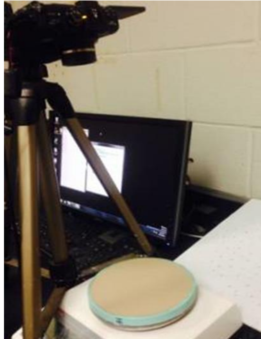
Figure 4.3 The experimental set up of desiccation tests
