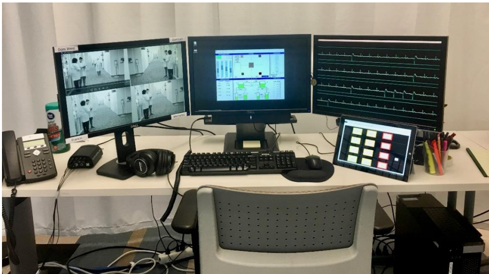
Figure 4-5: The simulation setup, distributed across three separate desktop monitors and a touchscreen tablet. Left to right: simulated surveillance video of the constructed Ardoin White hospital wings, the MATB-II display, the simulated physiological data display, and the charting display (touch screen).
