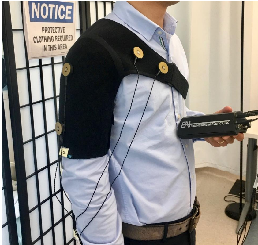
Figure 4-3: Arrangement and approximate location of the vibrotactile devices on the upper arm.
