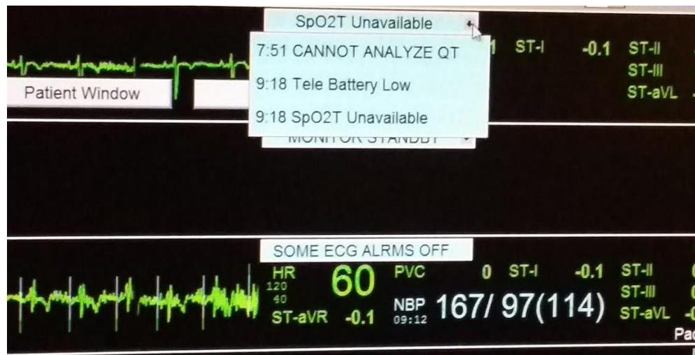
Figure 3-2: A sample view of multiple visual alerts appearing as messages in a displayed alarm box at the top of a patient’s window.
