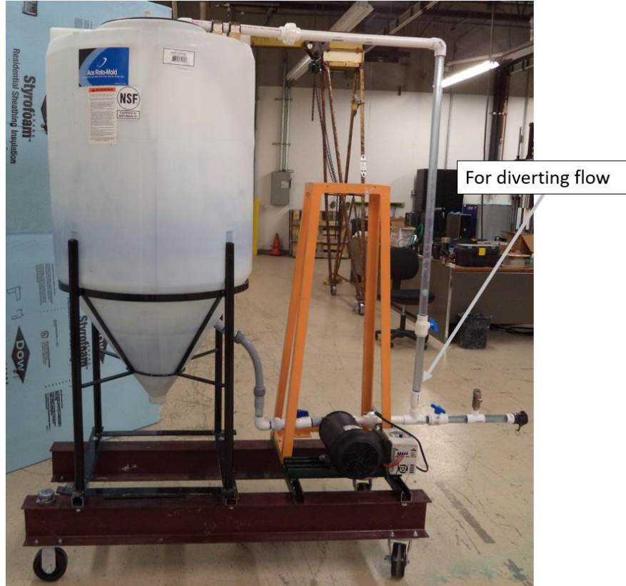
Figure 13. The Mixing Tank, Pump, VFD and Other Equipment
