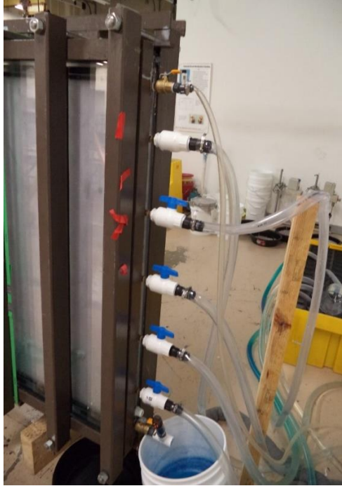
Figure 8. The Outlet Side of the Panel With Pressure Sensor
