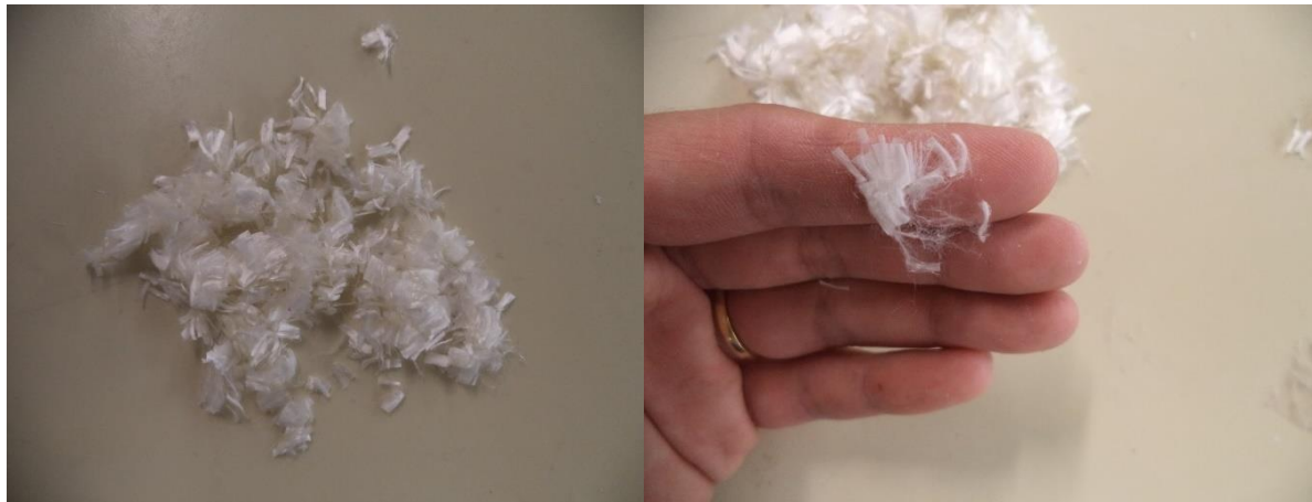
Figure 21. PGA/PLA 50/50 Fibers Still Maintained Fibrous Form
