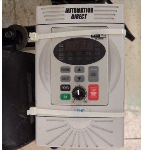
Figure 10. Automation Direct GS2-22P0 Variable Frequency Drive
