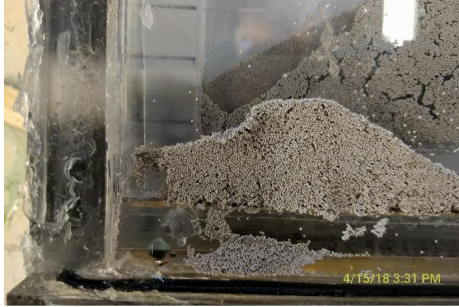
Figure 56. Dunes Between Panels
