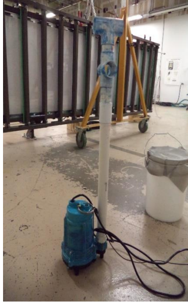
Figure 14. Submersible Pump for Circulating Slurries
