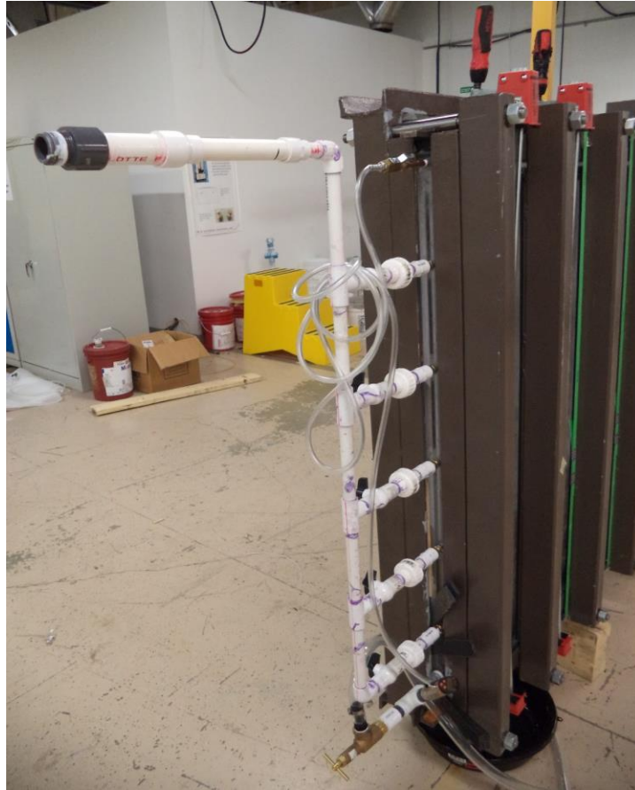
Figure 7. The Inlet Side of the Panel With Inlets and Pressure Sensor
