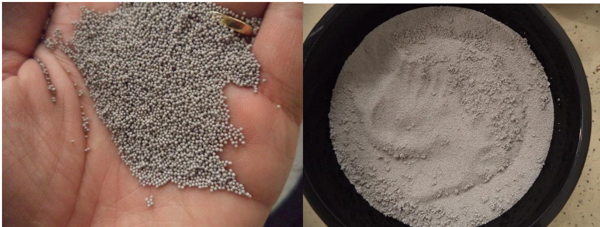
Figure 19. CARBO Proppant With Mesh Size 20/40
