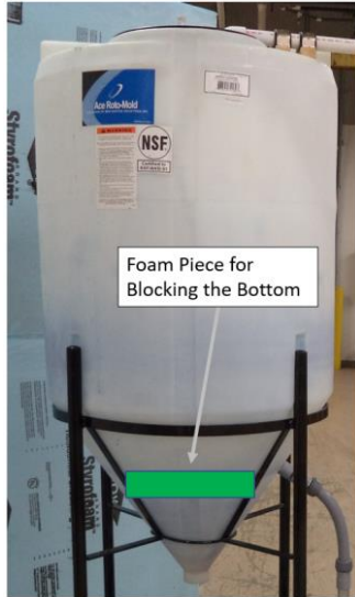
Figure 83. Location of the Foam Piece in the Mixing Tank
