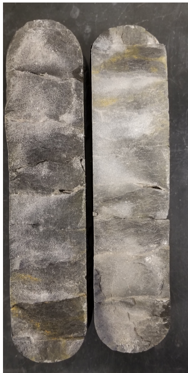
Figure 4.10: Fracture surface top and bottom, note the white coloration of the fracture surface due to sand crystals adhered to rock after sample cleaning.
