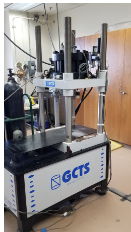
Figure 2.7: GCTS load frame used to apply closure stress for experiments.
