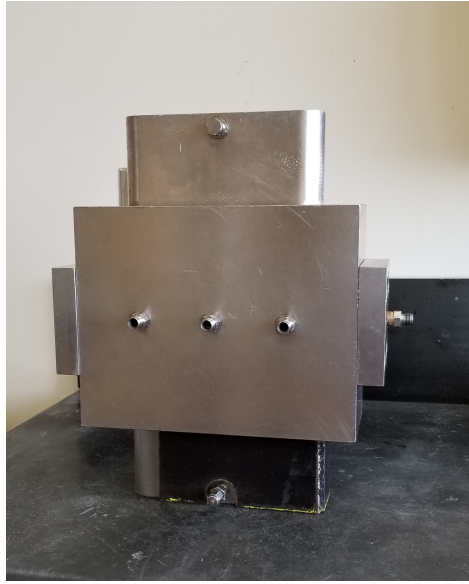
Figure 2.14: Completed conductivity cell assembly with sample placed inside.
