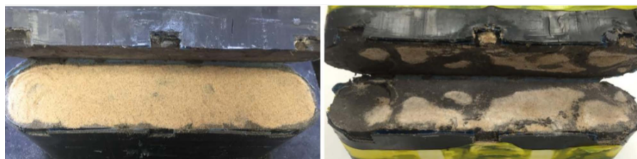
Figure 4.4: Left image is initial proppant loading of sample, followed by channeling effect seen in picture on right. Reprinted from Guerra et al. (2017a).
