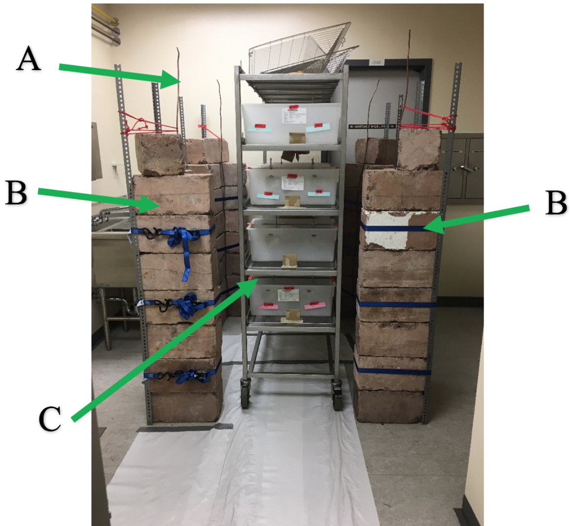
Figure 2.3 Pictured is the radiation field from the perspective of the door. A) Copper tubing which encases the active \text{Co}^{60} wires. B) On the left and right are stacks of nuclear shielding grade concrete blocks. C) Cart containing animal cages.
