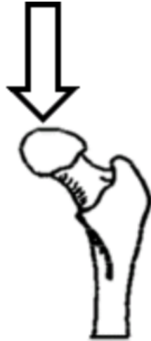
Figure 2.5 Left femoral neck compression test experimental setup (Artwork printed with permission from Jeremy Black).
