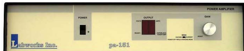
Figure B.3 Labworks pa-151 linear power amplifier.
