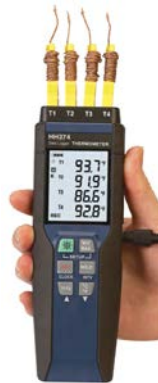
Figure B.13 OMEGA HH374 4-channel data logger thermometer.
