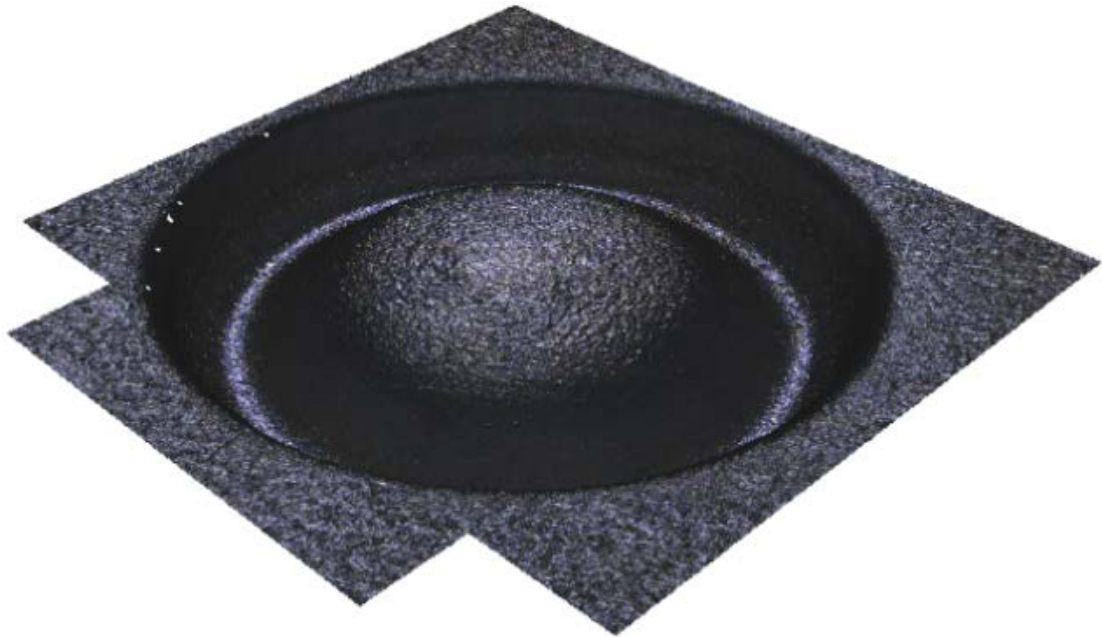
Figure 7.21 Resulted profile of an ECM'd hole.
