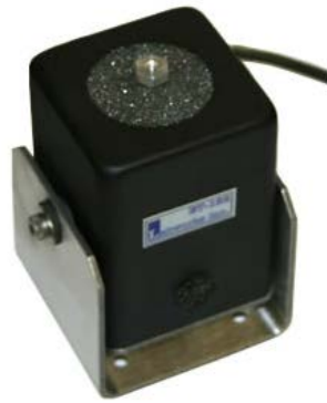
Figure B.4 Labworks ET-132 electrodynamic shaker.
