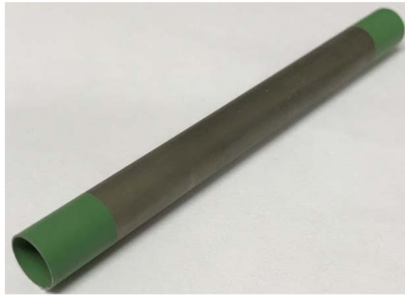
Figure B.14 Stainless steel cathodic electrode with Teflon coating.
