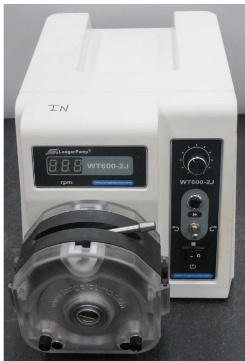
Figure B.10 Longer WT600-2J high flow rate peristaltic pump.
