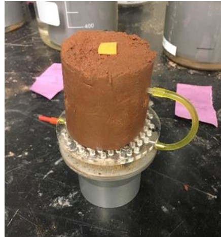
Figure 4. Soil core prepared for the TypoSoil machine
