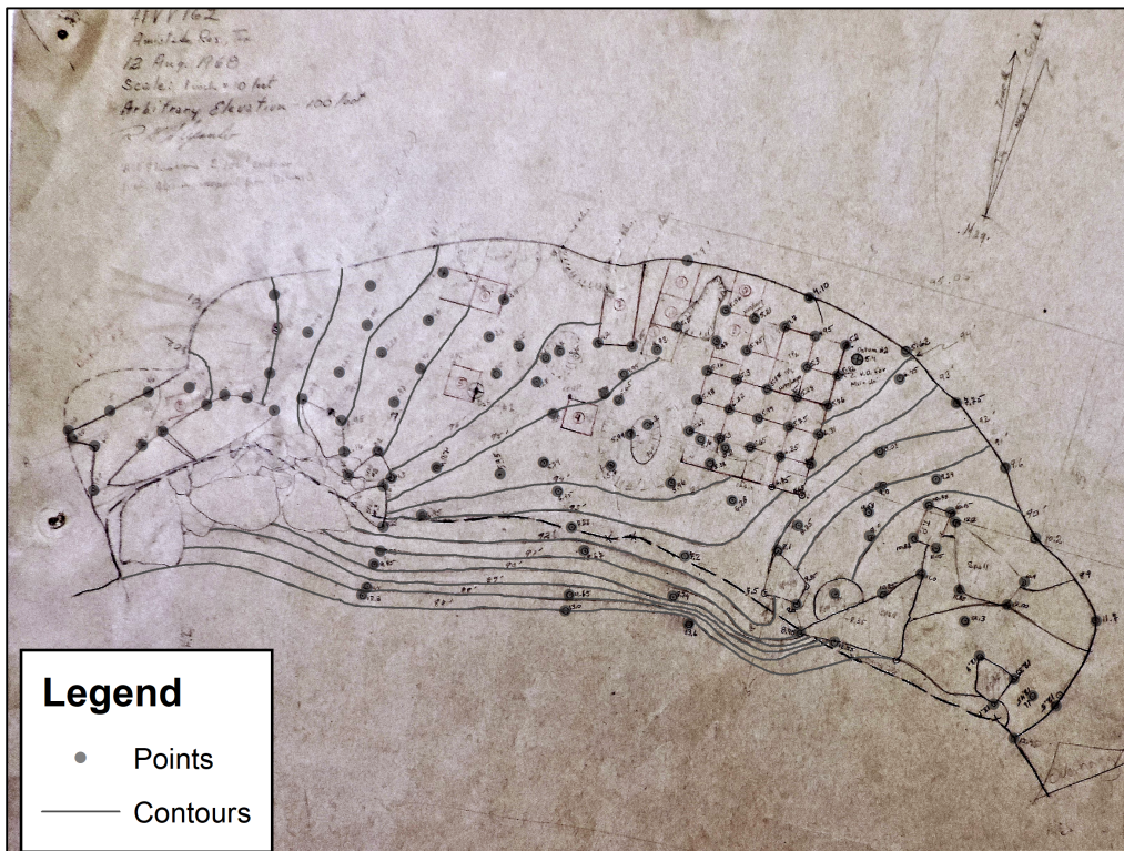
Figure 11. Plan map of Conejo Shelter showing digitized theodolite points and elevation contours. Image generated in Esri ArcGIS 10.3.
