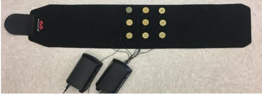
Figure IV-3. The spatial configuration of vibrotactile actuators on the belt
