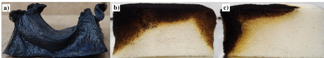
Figure 3.7 Cross sectional images of 5 BL BPEI/PAA (a), 3 BL HNT (b), and 5 BL HNT (c) coated PUF after 10 second exposure to a butane torch.
