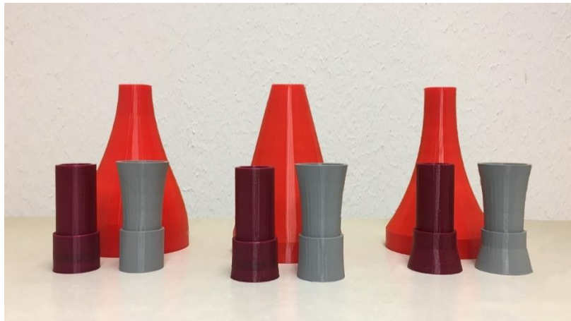
Figure 9: 3D-printed nozzle-forms ( L-R: 3, 4, 5 ) with their extensions, control (maroon-colored) and outwardly curved (grey-colored).
