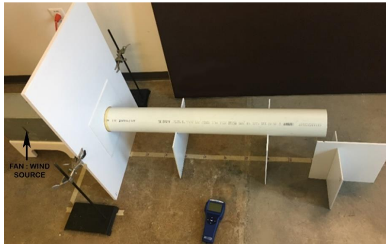
Figure 14: Apparatus used to investigate impact of tube lengths on wind-velocity output.
