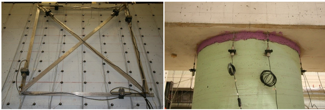
(a) Phase I Joint Region LVDTs
