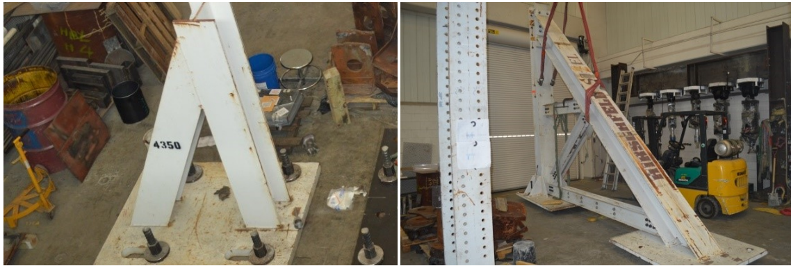
(a) Bottom Horizontal Actuator (HB) Reaction Frame
