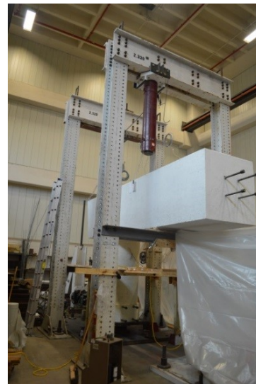
Figure 3.11. Vertical Reaction Frame. (Adapted with permission from Birely et al. 2018a)
