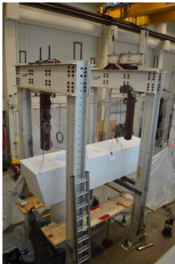
Figure 3.11. Vertical Reaction Frame. (Adapted with permission from Birely et al. 2018a)
