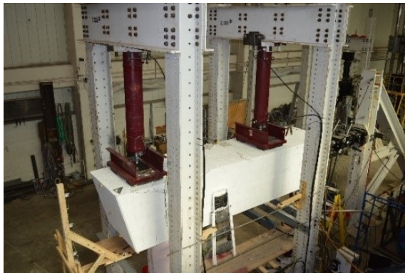
(b) Vertical Actuators Installed
