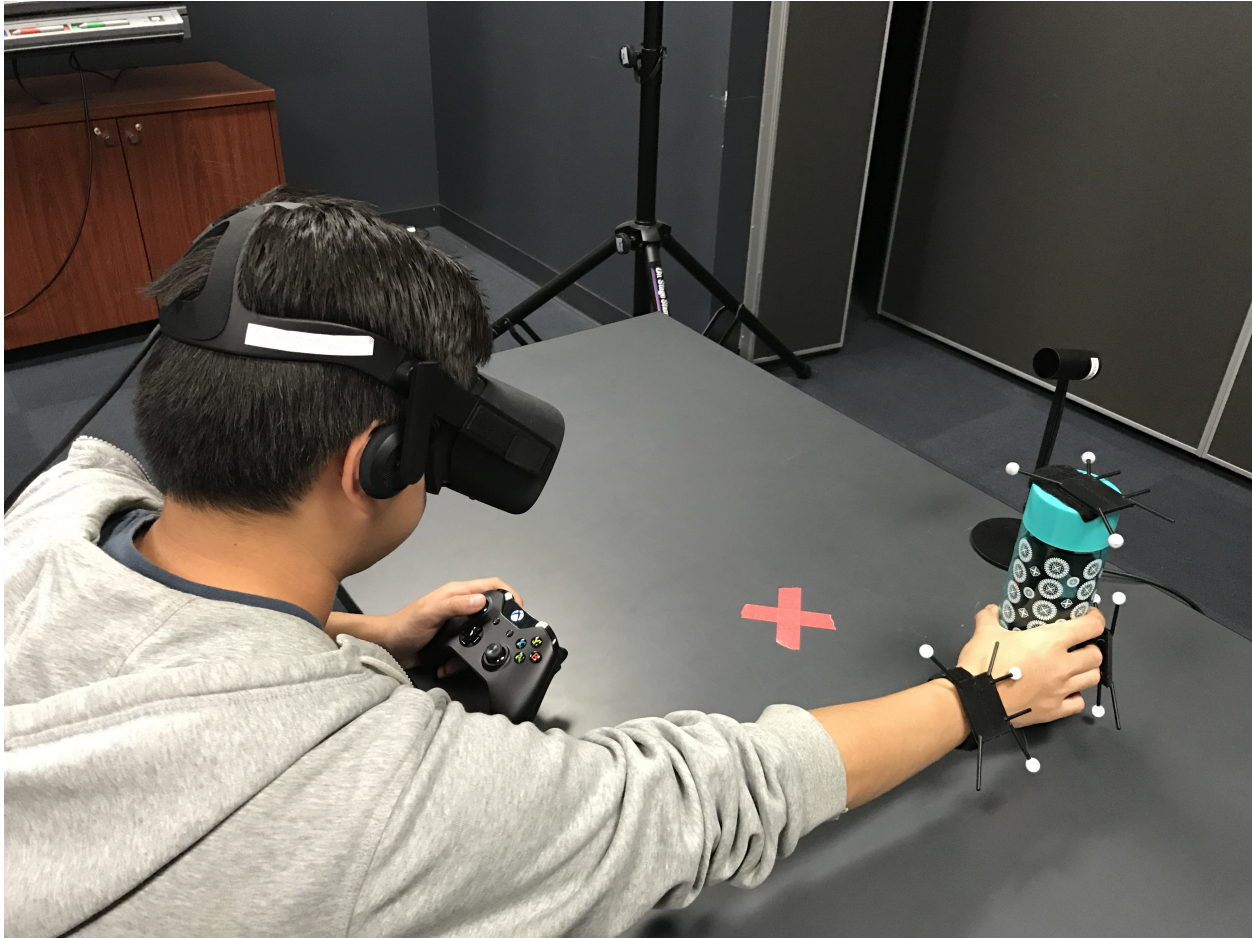
Figure 4.5: The physical setup used for the game study. Participants sat at a table and could reach and move a tracked prop (a plastic bottle). Tracking markers were placed on the wrist and fingers of the user’s right hand, and the left hand was used to operate the analog stick of a game controller. Participants could rotate in a swivel chair [31].
