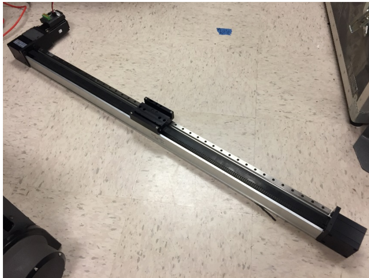
Figure 7 – Linear slide coupled with one of the stepper motors.
