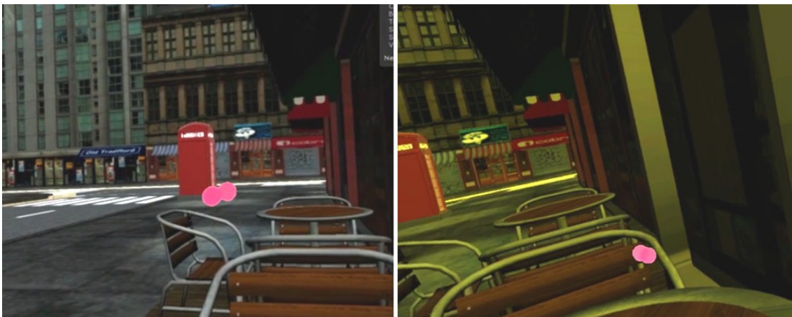
Figure 3.4: The full-image effect dynamically changes the rendered image in real time as the viewer looks away from the POI. The pink circles represent viewer binocular gaze.
