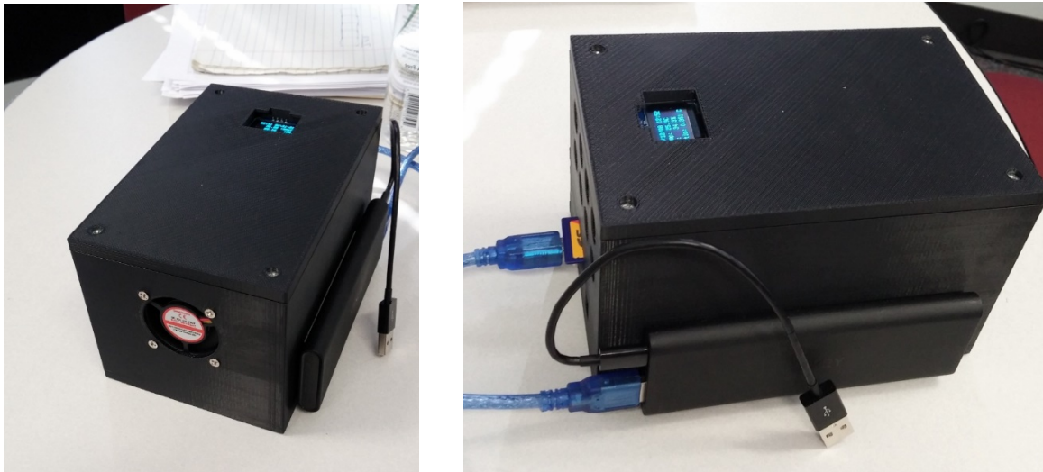
Figure 2-1. Custom Build Low-Cost PM2.5 Monitor
