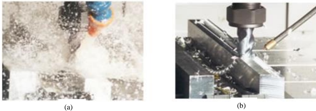
Figure 1 Machining with (a) Flood Cooling (b) Minimum Quantity Lubrication (Reprinted from UNIST Coolubricator, n.d.)
