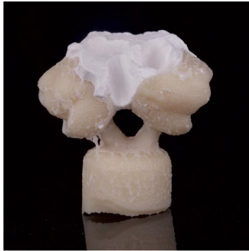
Figure 21. Fine removal of investment material at 30 psi with polishing beads.
