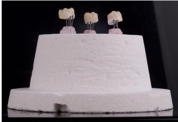
Figure 25. Cooled CAD crowns after the firing cycle.
