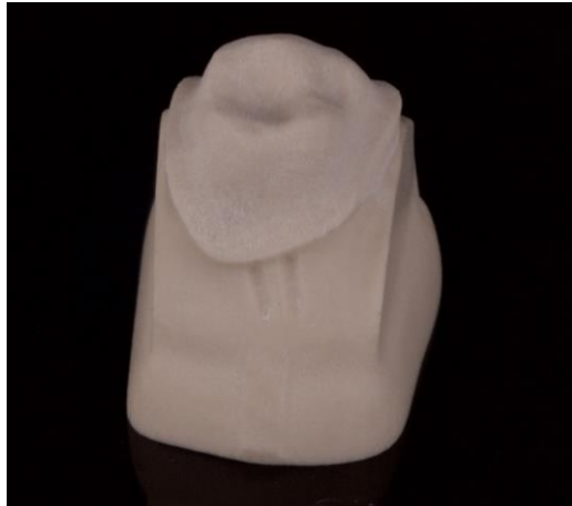
Figure 2. Milled epoxy resin 'Master Die'.
