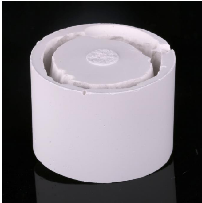
Figure 20. Gross removal of investment material at 60 psi with polishing beads.
