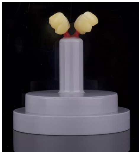
Figure 10. Two Ivoclar Vivadent ProArt CAD Wax milled crowns sprued to a ring base.
