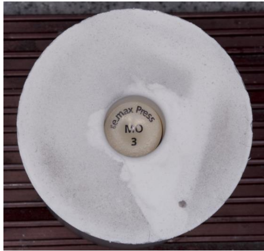
Figure 17. Investment ring with ingot inserted.
