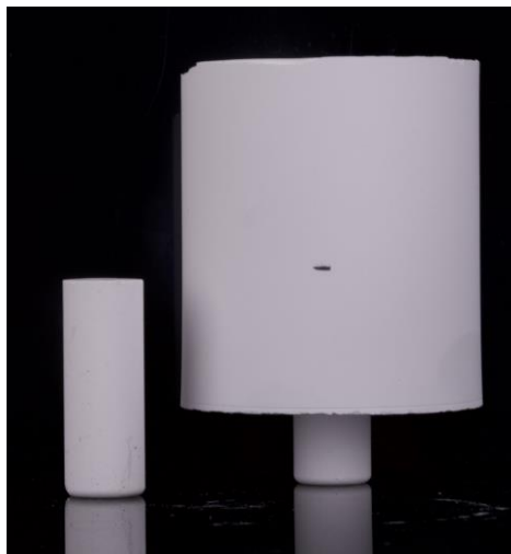
Figure 19. Single use plunger used to mark investment ring.
