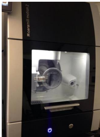
Figure 5. Amann Girrbach Ceramill Motion 2 5-axis milling unit.
