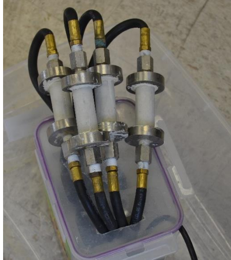
Figure 34 – Healing Rig – comprises of a reservoir of the healing water which is pumped through the pipe section specimens by a submersible pump at a flow rate of 0.6 m/s.
