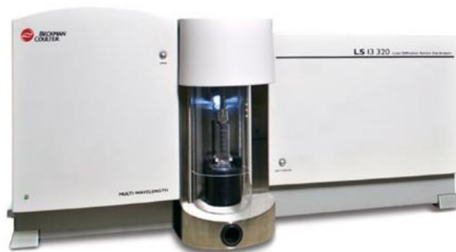
Figure 27. Beckman Coulter LS 13 320 particle analyzer
