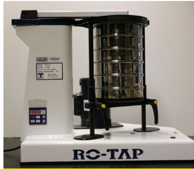
Figure 39. TAMUQ mechanical sieve (RoTap RX-29 Sieve-Shaker)
